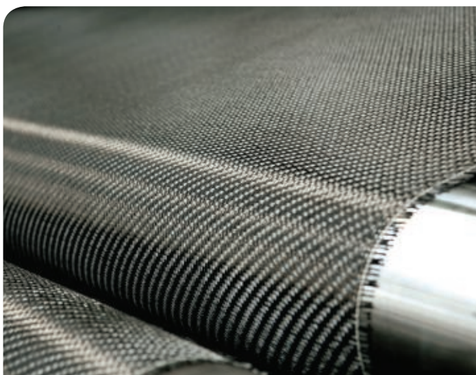
Left: Carbon fibre reinforced plastic is extremely light and resilient and reduces the weight of the aircraft by almost 20 per cent
